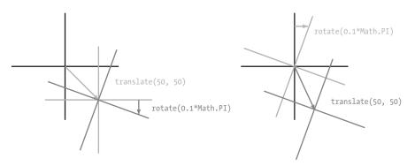
But if we *first* rotate by 20 degrees and *then* translate by (50,50), the translation will happen in the rotated coordinate system and thus produce a different orientation. The order in which transformations are applied matters.
