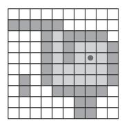
The flood fill does not leak through diagonal gaps and does not touch pixels that are not reachable, even if they have the same color as the target pixel.
